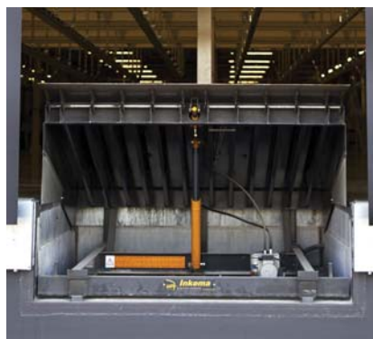
Lifting cylinder with anti-fall valve
