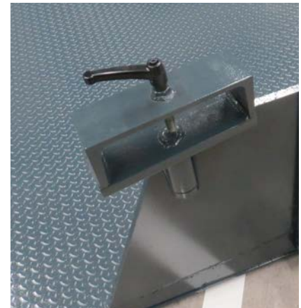
Forklift blade fastening for directing the ramp
