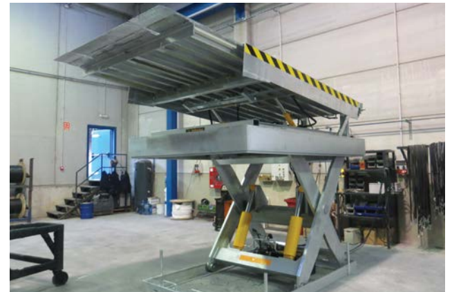
Galvanised Dual Scissor Lift Table with 1000mm telescopic lip.
