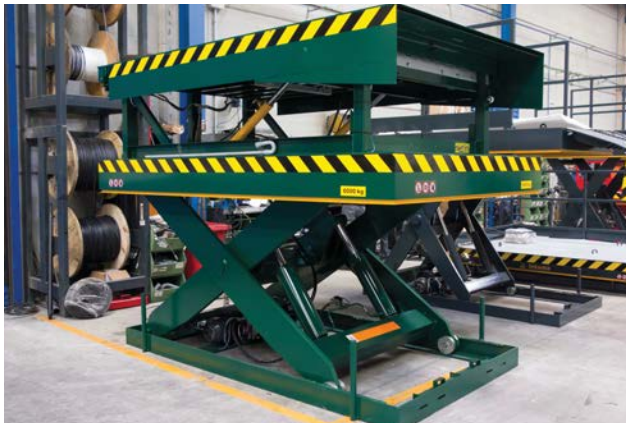
Dual Scissor Lift Table with 500mm telescopic lip.
