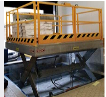
Galvanized table with hinged doors, side rails and interlock.
